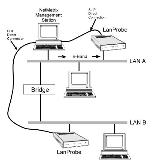
Figure 1-2: LanProbe System Example
